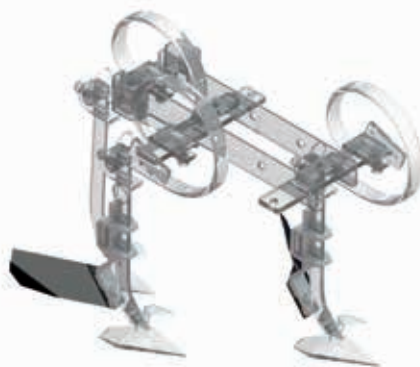
Heaping shares are used for hilling up the plant rows. They can be mounted on the holder of the vibrotine as well as on the Danish spring tine.
