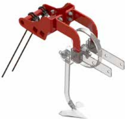
Adjustable weeder tines for CHOPSTAR 20-30 cm / 7.9-11.8", CHOPSTAR 25-59 cm / 9.8-23.3" and CHOPSTAR 60-90 cm / 23.6-35.4". The outer tines on each section can be turned around, in order to push soil away from or towards the row (not on CHOPSTAR 20-30 cm / 7.9-11.8").
