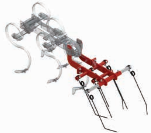
Adjustable weeder tines for CHOPSTAR 20-30 cm / 7.9-11.8", CHOPSTAR 25-59 cm / 9.8-23.3" and CHOPSTAR 60-90 cm / 23.6-35.4". The outer tines on each section can be turned around, in order to push soil away from or towards the row (not on CHOPSTAR 20-30 cm / 7.9-11.8").
