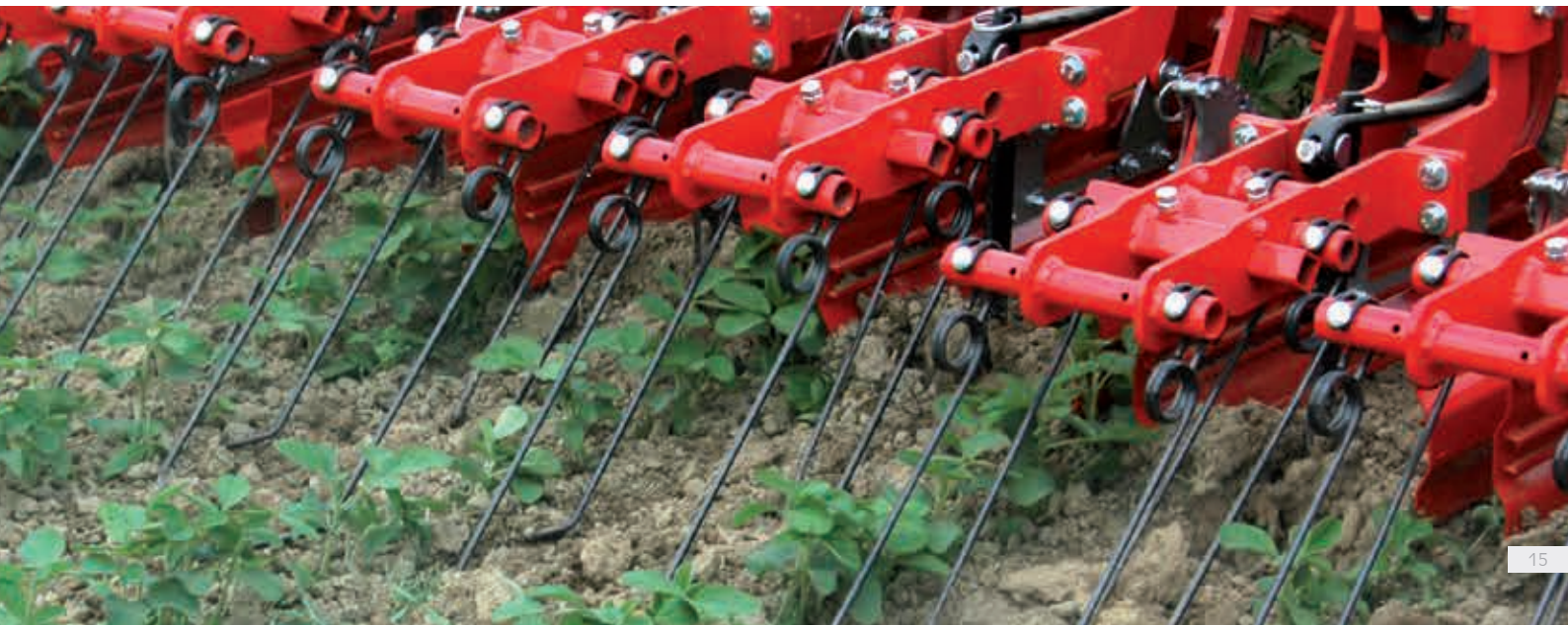
Hoe section CHOPSTAR 25-59 cm / 9.8-23.3", with hinged crop protection shields and vibrotines for shallow operation
