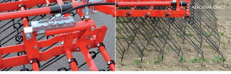
The **hydraulic tine adjustment** will make using the AEROSTAR-EXACT in changing soil conditions a whole lot easier. It also puts the tines in a flat angle when the AEROSTAR is folded.
