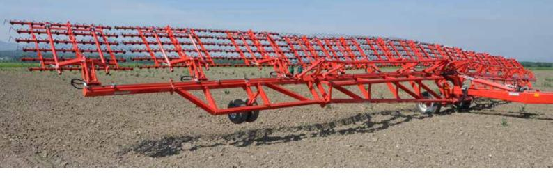
All sections of the semi pull type version of the AEROSTAR are attached to suspend beams. These beams are hydraulically controlled (hydraulic level adjustment).
