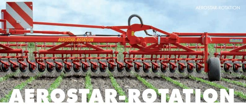
Rotating working tools unroot or cover weeds, encourage tillering and crack even hard soil crusts without any problems. The star wheels are **mounted inclined**, therefore the efficiency of weed control is outstanding.
