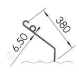
The tine with a diameter of 6.5 mm / 0.26" and a length of 380 mm / 15" is particularly suitable for **medium soil.**
