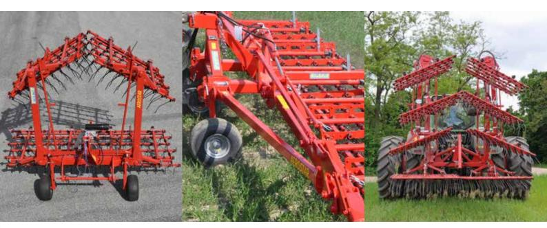
Folding the side sections will reduce the width of the AEROSTAR to a **transport width of only** 2.6 m to 3 m / 8.5 ft to 9.8 ft. Larger working widths, especially with shear retraction, are made possible through a large **angular support brace** that will keep the frame from swinging even at higher speeds and aggressive tine position.
