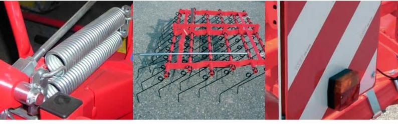
Implements with a working width of 4.5 m and 5 m / 14.8 ft and 16.4 ft fold manually or hydraulically and are **spring supported.**
