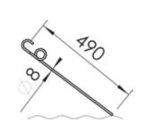
For **rocky soil** we recommend this straight tine so that the rocks are not moved to the surface. It has a diameter of 8 mm / 0.32" and a length of 490 mm / 13.9".
