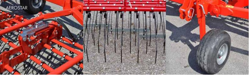
The **hydraulic tine adjustment** will make using the AEROSTAR in changing soil conditions a whole lot easier. It also puts the tines in a flat angle when the AEROSTAR is folded. Small molehills can be levelled by **grassland plates** which are mounted directly to the tines.
