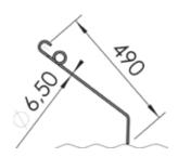
The tine with a diameter of 6.5 mm / 0.26" and a length of 490 mm / 19.3" is designed for **very light soil conditions.**
