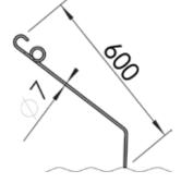
This tine with a diameter of 7 mm / 0.28" and a length of 600 mm / 23.6" is well suited for **special crops**. It also compensates for **uneven soil** very well. This is the least aggressive tine offered.
