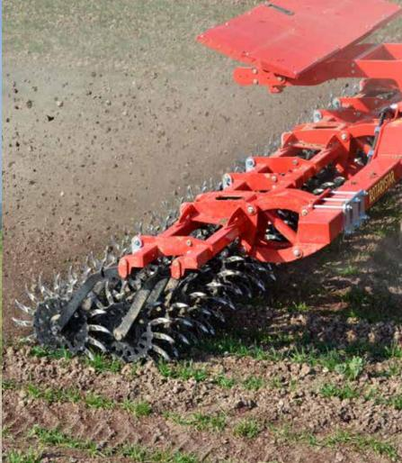
The hydraulic folding allows a transport width of only 3 m.
