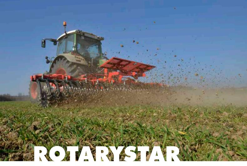
Due to the rolling motion of the rotor stars no plant residues are collected – ideal to **fight weeds in mulch-till crops**.
